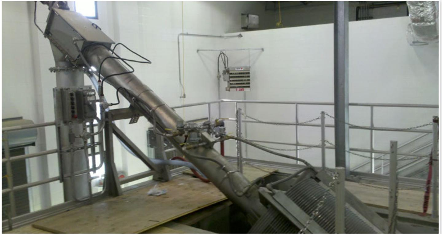
The In Channel Drum Screen is suitable for treating flow rates up to 45 mgd per screen.
