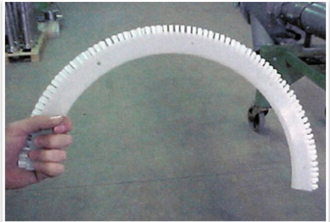
Easily Replaceable "Bolt On" Brushes.
